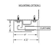
CONCRETE/FILLED BLOCK JAMBS USING 3/8" X 4" POWERS WEDGE BOLT
